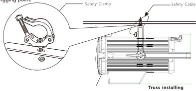
Regardless of the rigging option you choose for your PROFILE NF 200CWWW, always be sure to secure your fixture with a safety cable. The fixture provides a built-in rigging point for a safety cable on the hanging bracket as illustrated above. Be sure to only use the designated rigging point for the safety cable and never secure a safety cable to a carrying handle.
